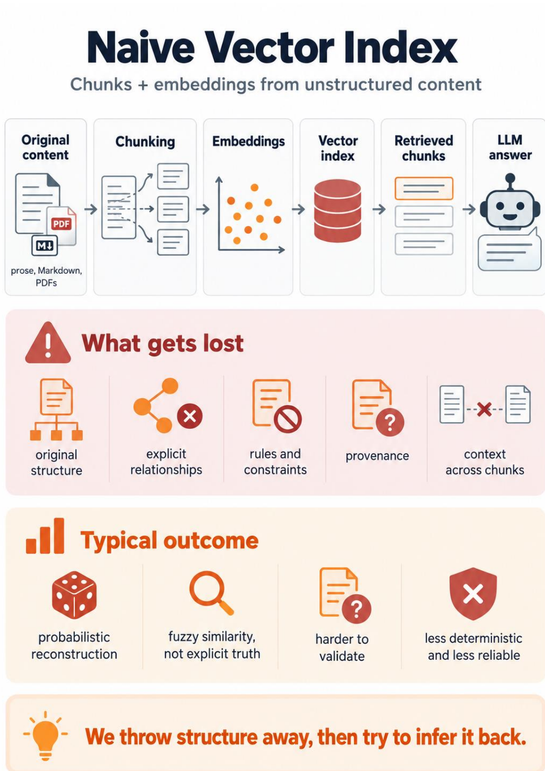
Figure 1. Conventional vector retrieval can weaken or lose explicit structure, relationships, rules, provenance, and cross-chunk context.
