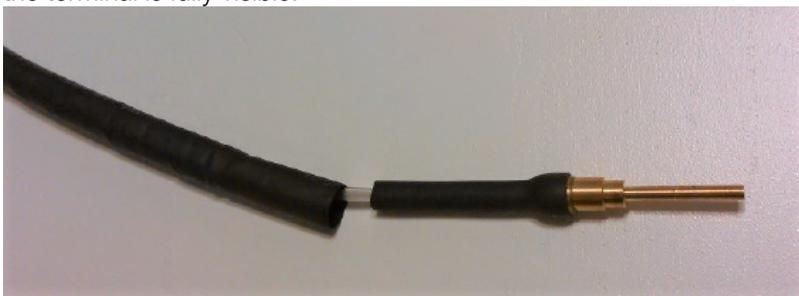
2. Place the tube so that it partially covers the small rubber section of the existing fiber terminal.
