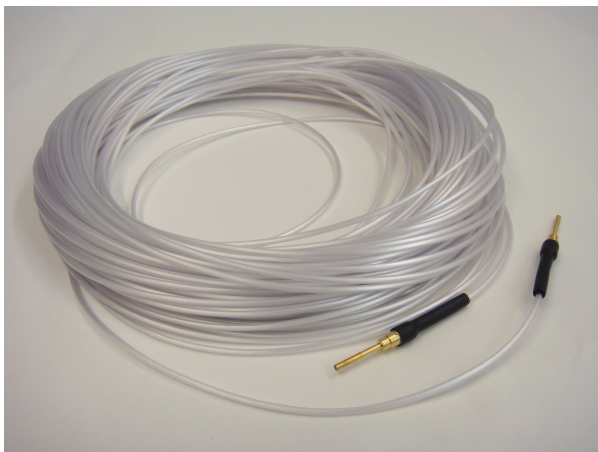
Figure. 5.4. - 16. AQ-07 sensor with covered ends.
