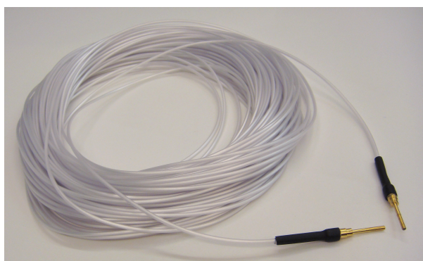
Figure. 5.5. - 17. AQ-08 sensor with covered ends and terminals.
