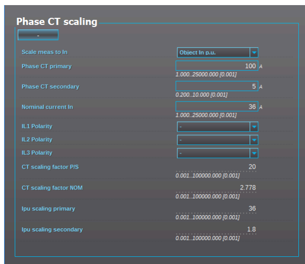
Figure. 4.2.1 - 5. Setting the phase current transformer scalings to the protected object's nominal current.
