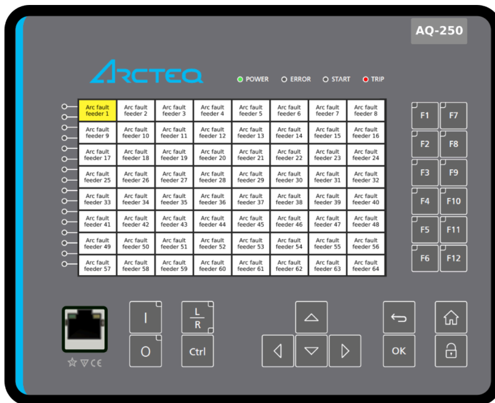
Figure. 5.6 - 27. In AQ-S254 it is possible to set up the display to show sensor activations in alarm display.
