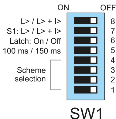
Figure. 4.4.2 - 9. The DIP switch settings for SS:0.
