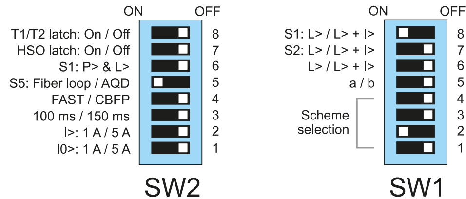
Figure. 4.5.2 - 26. The DIP switch settings for SS:2b.
