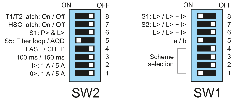
Figure. 4.5.2 - 17. The DIP switch settings for SS:1a.
