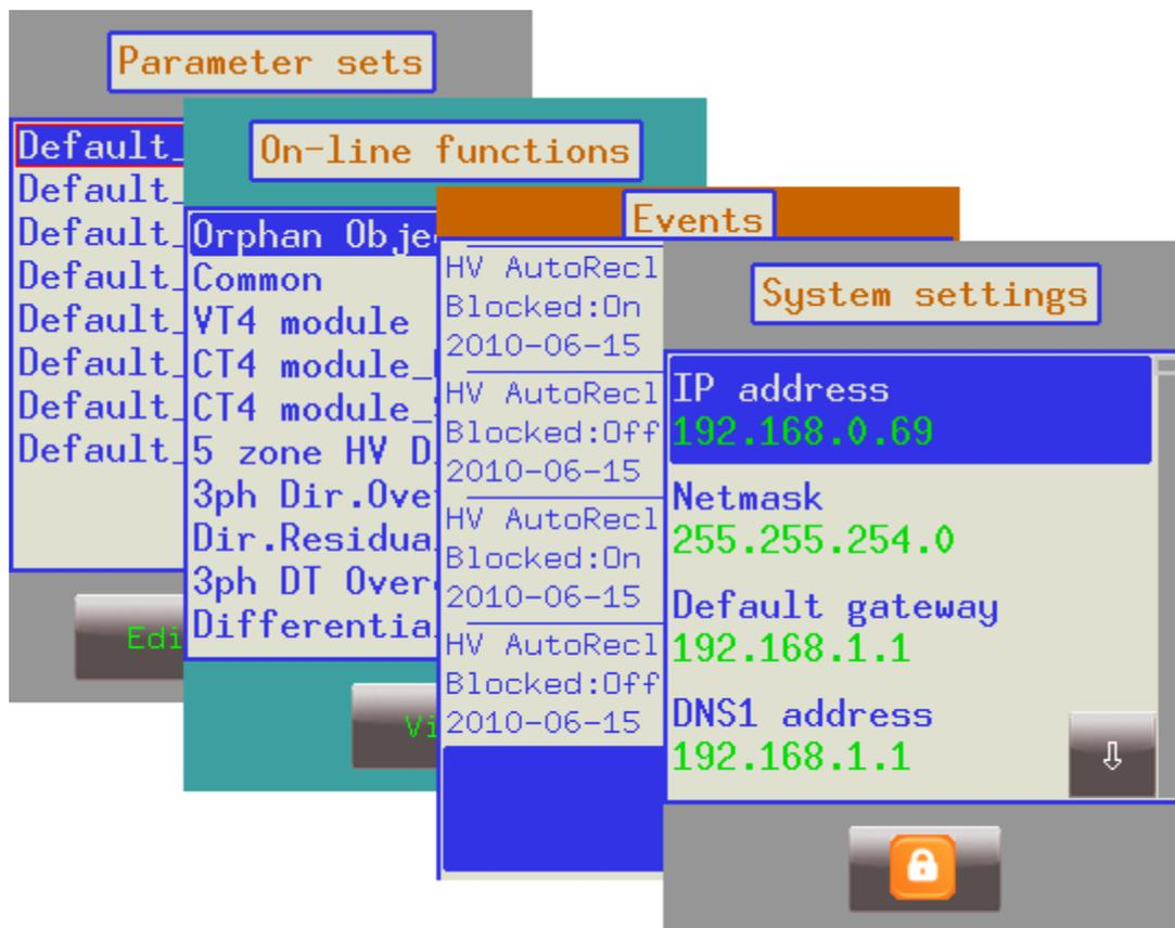
Figure 2-4 Some screens displayed on the LCD
