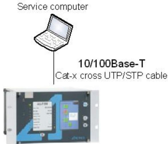
Figure 2-7 Using the RJ-45 connection to connect a computer directly
