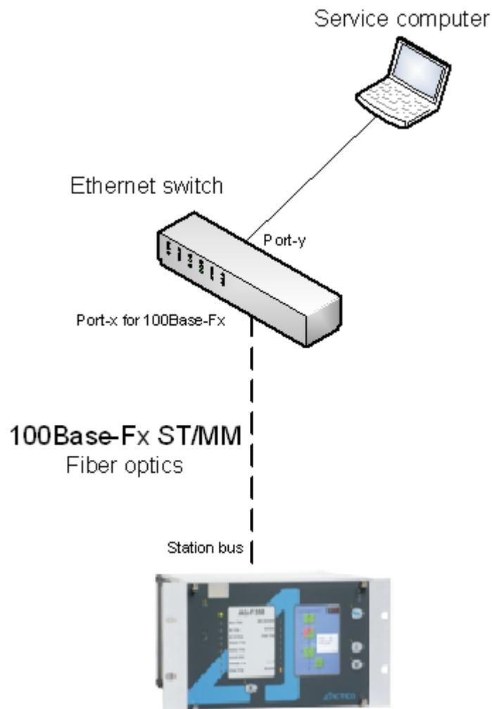
Figure 2-9 Using the ST type fiber optic connection to connect computers via optical Ethernet switch
