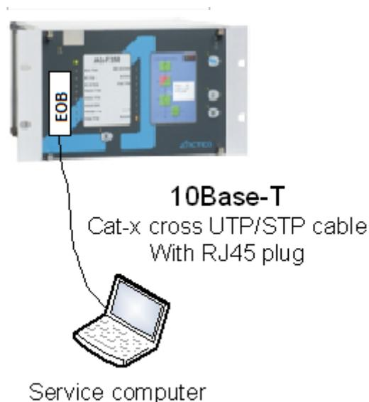
Figure 2-6 Using the EOB connection
