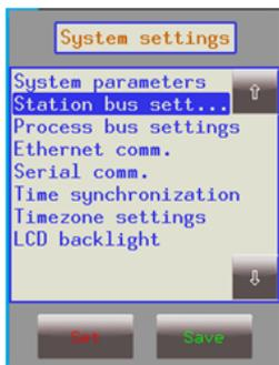
Select "Station bus settings" and press
