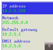
These addresses here define the Ethernet communication of the station bus. Here most important addresses are the IP address and Default gateway (if used). Also if DNS is used in the network it is set here.
