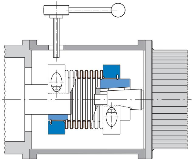
By applying clamping ring hubs, the smartflex®-steel bellows couplings can be mounted in areas which are difficult to access. Please provide an opening in the bell housing for the Allen wrench as depicted in the example.
