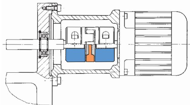
The ROBA®-ES shaft coupling transmits the torque backlash-free between the motor shaft and the output shaft. It also compensates for axial, radial and angular shaft misalignments.
