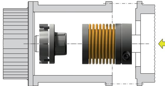
The primeflex®-steel bellows coupling transmits the torque backlash-free between the motor shaft and the gear shaft. By applying plug-in shrink disk hubs (see Installation Example) or plug-in clamping hubs, the primeflex®-steel bellows couplings can be mounted in areas which are difficult to access.
