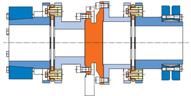
The measurement flange is positioned between the two disk packs. This way, the measurement flange can be de-installed radially with the sleeve, for example for calibration, without de-installing the hubs. Backlash-free shaft-hub connection via shrink disk hub or hub with external shrink disks ensures maximum precision.
