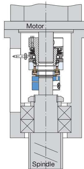
ROBA®-DS shaft coupling combined with an EAS®-torque limiter. Backlash-free and torsionally rigid torque transmission between the motor shaft and the spindle shaft. Compensation of axial, radial and angular shaft misalignments.
