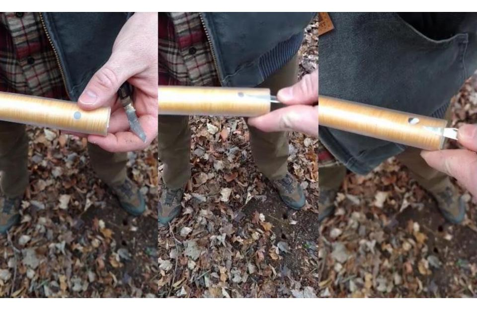
Use a small knife or spatula to separate the film from the edge of the tube so that the hook on the push rod can catch in the hole.
