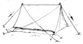
9. Peg out the other guy lines, corner ones first. Generally, if a corner has one guy rope it is pitched at 135 degrees or, if it has two, they are pitched at 90 degrees. The pegs should be placed so that the runner, when the guy line is taut, is about one-third of the way up from the peg. The side guy line pegs should be in a line parallel with the ridge pole and the guy lines following the tent seams.
