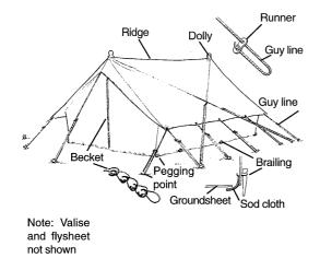
*Guy lines* - These may also be known as 'guys' or guy ropes'. A guy line is a single line or rope which comes from a part of the tent which, when the tent is pegged into the ground and when the guy line is pulled tight, creates the familiar tent shape. Badly tensioned lines cause a tent to sag and when raining, pockets of water form which may then drip into the tent. These lines also help to keep the tent down in high winds.
