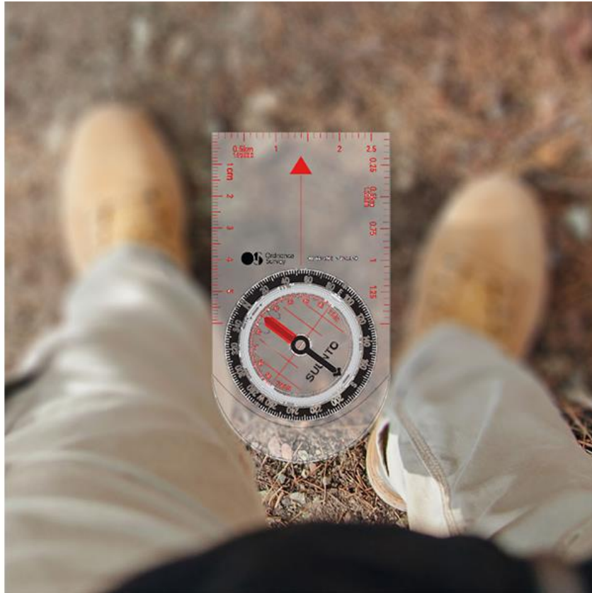
Compass bearings step 3: adjust for magnetic variation
