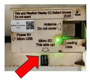
**IMPORTANT:** Images shown are for the 2.8 inch version of the display. The 7 inch and 5 inch display backside looks like this (note the different locations for the SD Card and Power):
