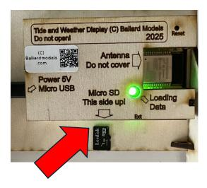
You can remove the card by pushing on it, it is loaded with a little spring and will push out a little. To remove it completely you can use tweezers or a little screwdriver to pull it out. Insert it into your SD card reader on your computer. On the card, you will find the Config.cfg file. Open it with a text
