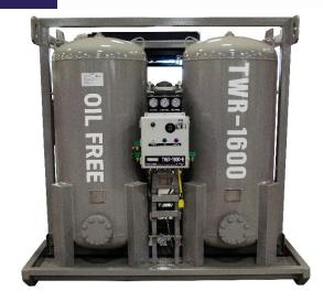
Designed for the rugged demands of the oil-free rental industry. DryAire Rentals Oil-Free TWR Series, delivers clean, dry oil-free air, all in one complete, reliable package. Skid package includes an air cooled after cooler, bulk moisture separator, coarse pre filter, fine pre filter, heatless regenerative desiccant dryer and particulate after filter.
