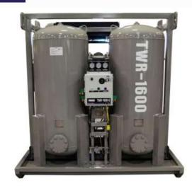
Designed for the rugged demands of the rental industry. DryAire Rentals TWR Series, delivers clean, dry air, all in one complete, reliable package. Skid package includes an air cooled after cooler, bulk moisture separator, coarse pre filter, fine pre filter, heatless regenerative desiccant dryer and particulate after filter.
