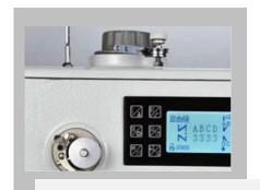
Dial for easy adjustment of sewing foot alternation up to 5.5mm. Improved bobbin winder for
