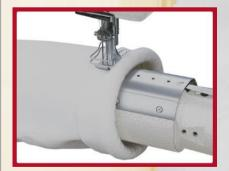
Mauser Spezial MA0269-273 two-needle machine in a filter processing application.
