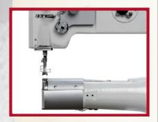
75mm diameter of the cylinder arm in the sewing area and arrangement of the sewing tools for sewing close to the edge.
