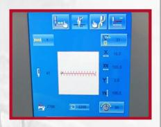
LCD touch control panel for easy programming and adjustment of the bartack parameters.
