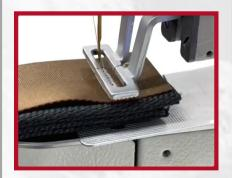
Very high lift of the clamps for inserting up to 1" of webbing material (special conversion for the parachute industry).
