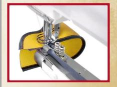
Standard version of the Mauser Spezial MH1235. Footlift by knee switch, backtacking by hand lever.
