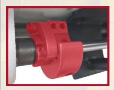
Safety clutch to prevent damage to the hook in case of excessive load.
