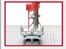
The asymmetric needle gauge is the perfect choice for smaller shops using only one machine for double and single needle operations. (Optional)
