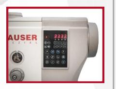
With the integrated 750W direct drive you can handle all kinds of sewing operations, while the integrated control panel allows easy access to the main sewing parameters.
