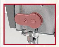
Integrated thread clamp for a clean seam beginning.
