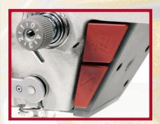
Favorite key for activating an intermediate bartack at the touch of a button without having to release the sewing material.
