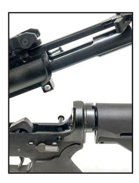
6. Remove the charging handle by pulling it backwards the keyway and then down and out of the upper receiver.
