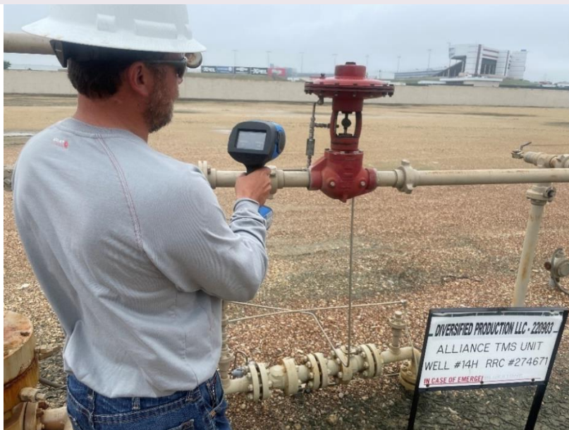
Figure 8: Demonstration of handheld emission detection device
