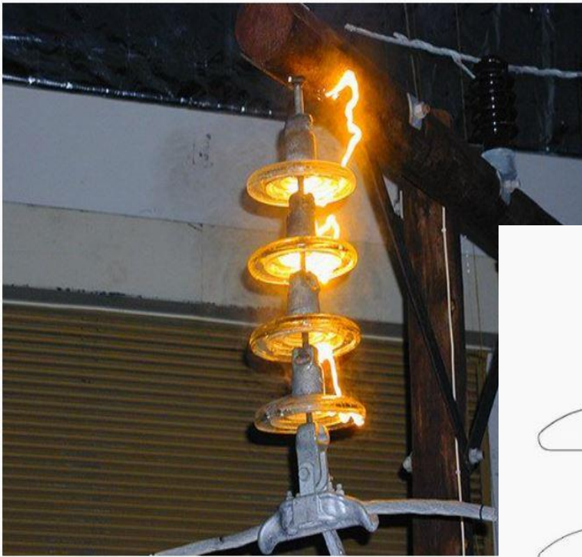
Power frequency dry flashover voltage test on insulator
