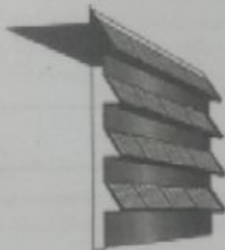
Building Integrated PV
