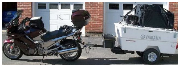
Bad example: Poor hitch, overloaded trailer
