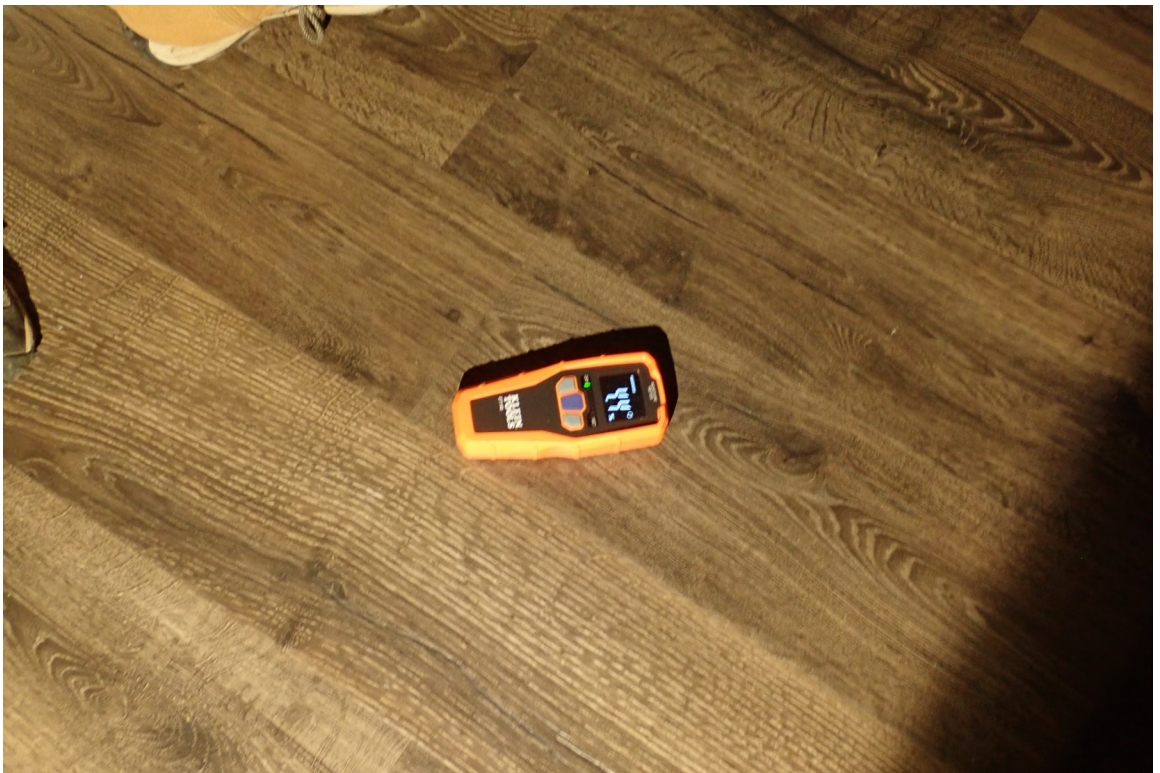
Figure 4 Concrete moisture reading at previous repair location
