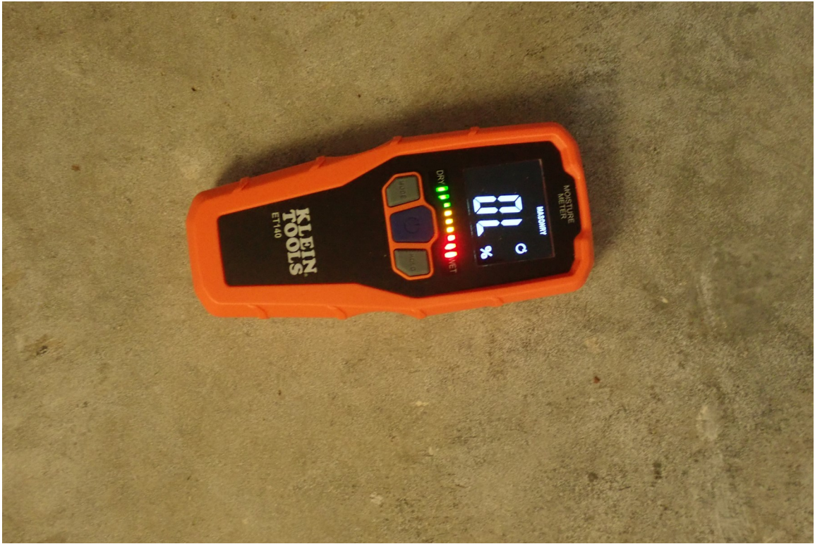
Figure 1 Concrete moisture reading inside
