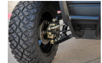
DOUBLE WISHBONE INDEPENDENT SUSPENSION
