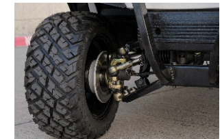
DOUBLE WISHBONE INDEPENDENT SUSPENSION
