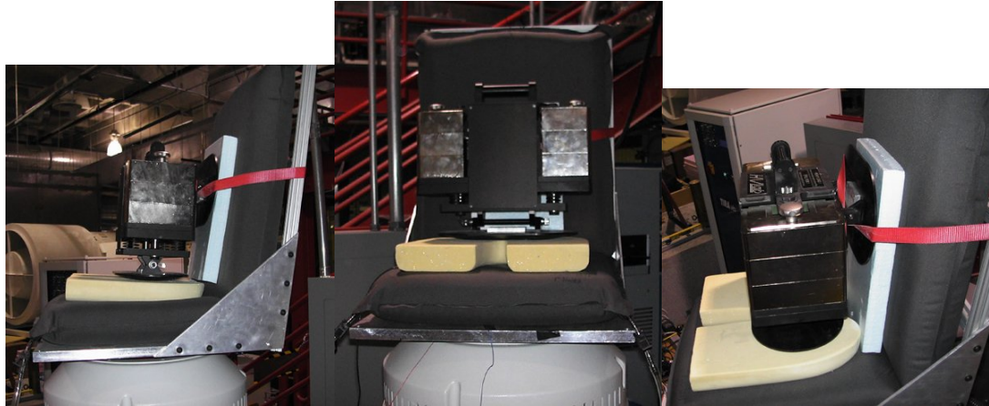
Figure 4.1 Experimental Setup for Seat Vibration Transmissibility
