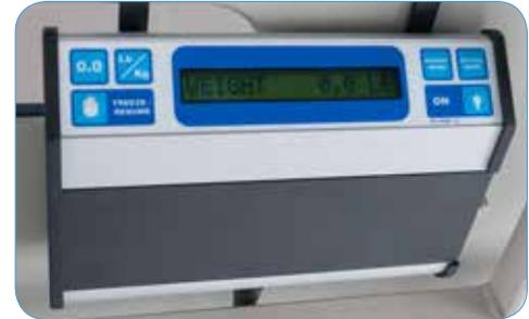
Optional factory-installed scale system
