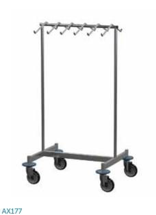
Lead Apron Rack 700 x 600 x 1420mm Stainless steel construction 12 apron hooks Corner buffers 125mmØ castors
