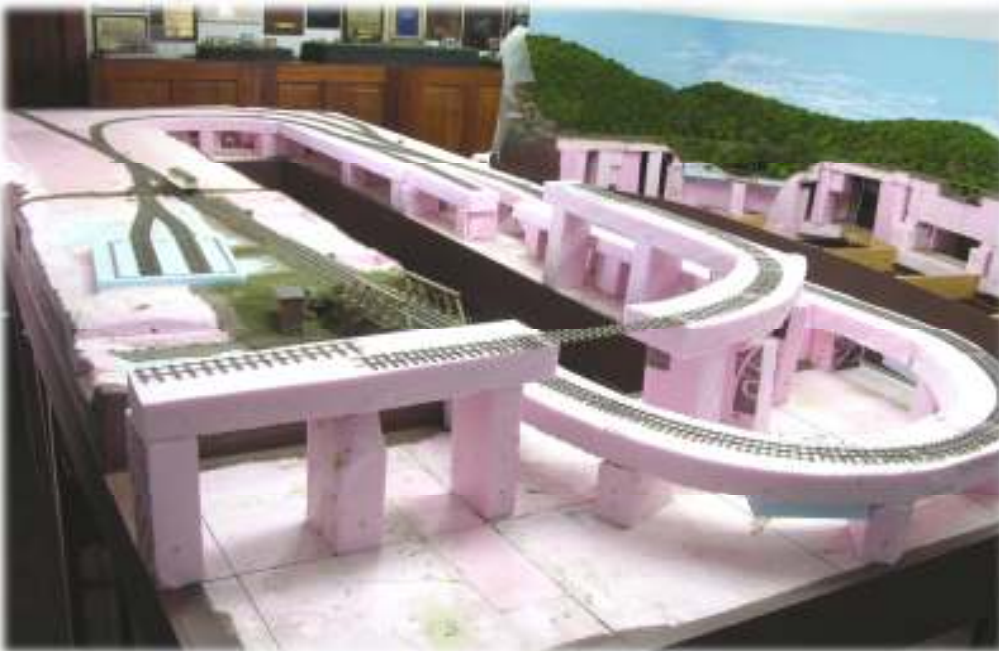
Beam and Column Roadbed
