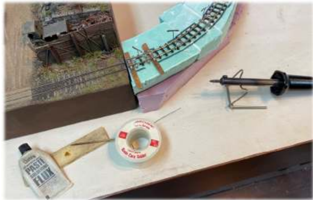
Printed Circuit Board Tie Soldering
