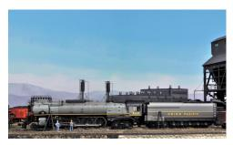
(Cover Photo): This is an Athearn Genesis 4-8-4 It was in very poor shape when I purchased.it. I added the missing details and had to scratchbuild a few parts. The oil bunker was backdated to match an in-service locomotive. I ended up converting it from an FEF-3 to an FEF-2 and gave it a complete paint job, in the Two Tone Gray scheme. Now she stays busy pulling passenger trains on the Denver Pacific.
