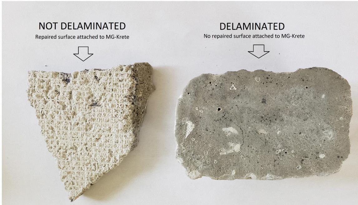
The first picture is that of MG-Krete attached the substrate, which would not be considered a failure. The second picture shows MG-Krete coming off the repaired substrate clean with none or less than 30% of the substrate attached, which would result in Imco Technologies supplying the repair material to fix the affected areas.
