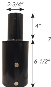
PRPT3 (3") PRPT4 (4") Tenon adaptor, 3" or 4" round pole, to standard tenon, bronze
