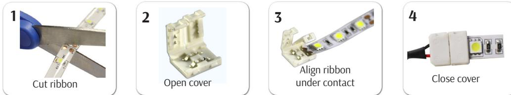
\* IP54 and IP65 connections should be sealed with silicon sealer and covered with heat shrink.
