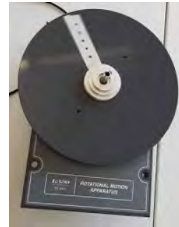
Figure 3. Commercially available lab turntable.
