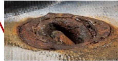
Separation bolt melting and erosion post-Artemis I reentry
