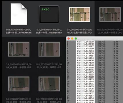
The image metadata contains the camera's intrinsic and extrinsic parameters and the status of RTK.
