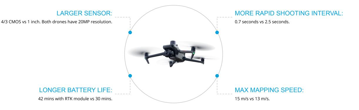
The Mavic 3E's larger pixel size (3.3 $\mu$ m vs 2.4 $\mu$ m) and intelligent low-light mode offer improved performance in dim conditions - extending the window to conduct drone surveys.
