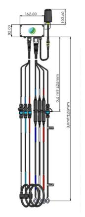
**Figure: Grid Data Logger with Detachable Accessories**
