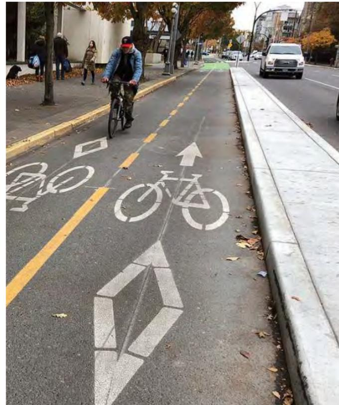
Example of a separated two-way cycle track.
