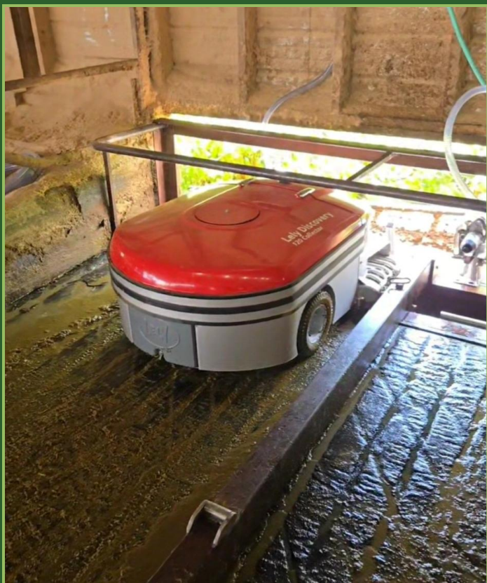
Lely Discovery 120 Collector, installed on the barn floor
