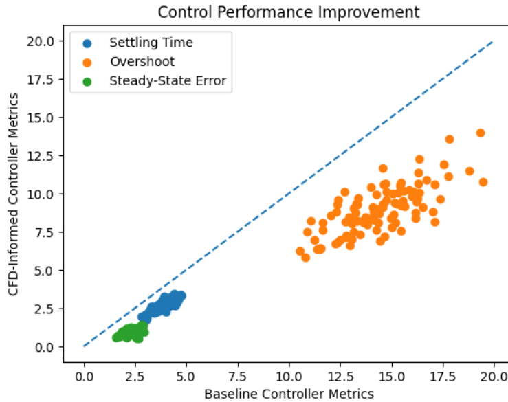
Fig. 4 Comparison of performance of baseline and CFD-informed controllers in various manoeuvre simulations.
