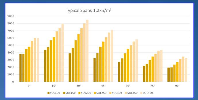
For each project Two Point Seven Facades Ltd will provide accurate sun angle calculations, based on the location of the site and orientation of the building, to determine the most efficient position, angle and pitch for your solar shading system.
