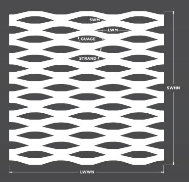
By inverting the expanded mesh panels they become more obscure. A chequer board effect can be achieved by rotating/inverting adjacent panels. Two Point Seven Facades Ltd offer a range of expanded mesh, with first class innovation, design and technical support to suit all applications. Email: info@twopointseven.co.uk
