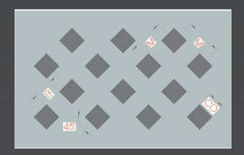
Square hole perforation, diagonal staggered pitch.
