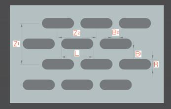
Slot hole perforation, rectangular pitch.
